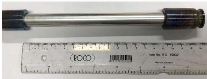
PdAu membrane after annealing under 31 bar pure H 2 at 550 °C for a total of 8.7 h.
